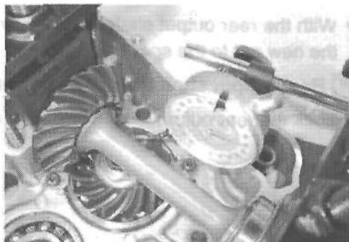
Measure the backlash by turning the drive bevel gear shaft in each direction, reading the total backlash on the dial gauge. If the backlash is not within specification, the shim must be changed and the backlash should be re-checked until correct. Refer to the chart at the right for appropriate shim thickness.
